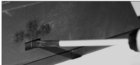
**Attention:** The wattage can be selected over a switch on the side of the device. Make sure that the selection corresponds to the wattage of the used lamp. Changing the wattage must only be done if the lamp is disconnected from power supply!
